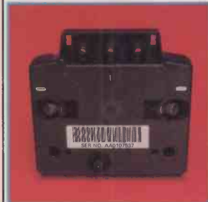
Because of its unusual geometry the Penman's body executes a curve even when drawing a straight line. The white slits are the paper edge detectors.
