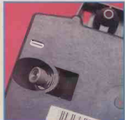
Because of its unusual geometry the Penman's body executes a curve even when drawing a straight line. The white slits are the paper edge detectors.
